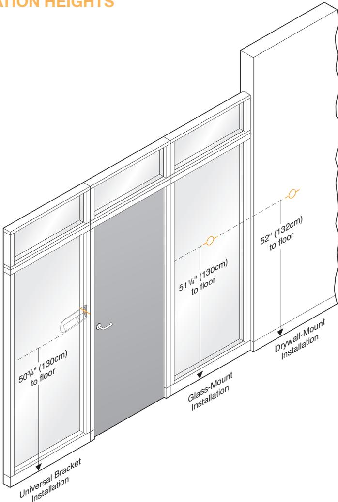
**ADA Accessibility Guidelines** require that the highest point of interaction not exceed 54 inches (137cm). For RoomWizard, this highest point of interaction is the top edge of the LCD screen. These installation instructions meet this 54-inch (137-cm) target height.
