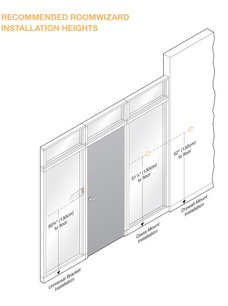
**ADA Accessibility Guidelines** require that the highest point of interaction not exceed 54 inches (137cm). For RoomWizard, this highest point of interaction is the top edge of the LCD screen. These installation instructions meet this 54-inch (137-cm) target height.
