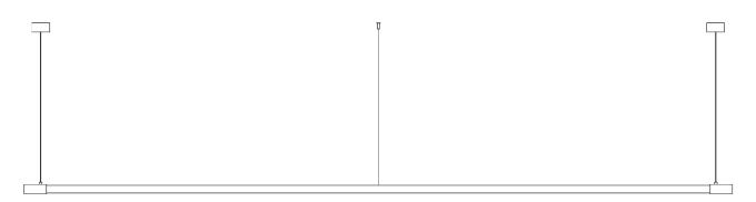
Dims: 2550 mm L, 40mm H, 30mm D Weight: 3.3kg
