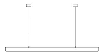
Dims: 1560 mm L, 72mm H, 54mm D Rose: 80mm dia x 38mm H Weight: 3kg
