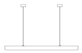
Dims: 1260 mm L, 72mm H, 54mm D Rose: 80mm dia x 38mm H Weight: 2.5kg
