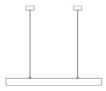
Dims: 960 mm L, 72mm H, 54mm D Rose: 80mm dia x 38mm H Weight: 2kg
