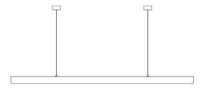
Dims: 1860 mm L, 72mm H, 54mm D Rose: 80mm dia x 38mm H Weight: 3.5kg
