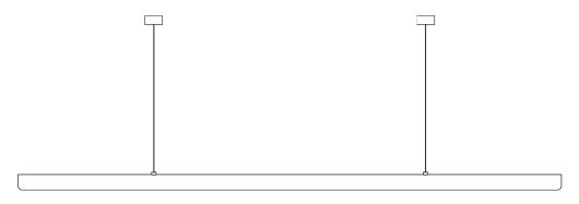
Dims: 2460 mm L, 72mm H, 54mm D Rose: 80mm dia x 38mm H Weight: 5kg
