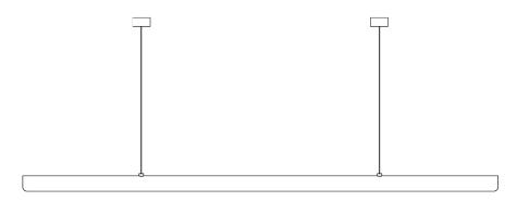
Dims: 2160 mm L, 72mm H, 54mm D Rose: 80mm dia x 38mm H Weight: 4kg
