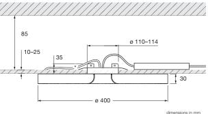
cover for revision can be ordered optionally (\*luminaire cable: 1 m)
