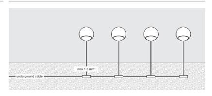
through-wired with plug in terminals
