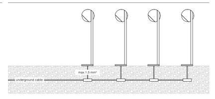
through-wired with plug in terminals
