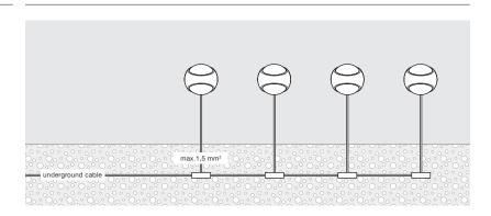
through-wired with plug in terminals
