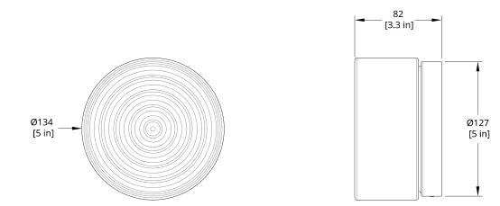
RP-WS Ripple Sconce Dimension (Rotate 90 degrees for flush mount version)
