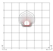
21.52 lm/W Efficiency Coordinate System Total Flux CG 170.03 lm Maximum Value 201.33 cd
