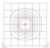
Efficiency Coordinate System Total Flux Maximum Value 88.00 lm/W CG 7154.22 lm 2122.35 cd
