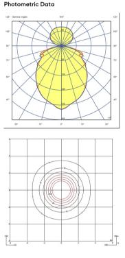
Efficiency64.98 lm/WCoordinate SystemCGTotal Flux1280.18 lmMaximum Value343.56 cd
