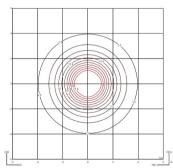
Efficiency 73.02 lm/W Coordinate System CG Total Flux 644.30 lm Maximum Value 259.03 cd
