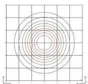
Efficiency Coordinate System Total Flux Maximum Value 38.65 lm/W CG 868.47 lm 348.73 cd
