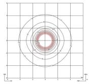
Efficiency Coordinate System Total Flux Maximum Value 78.79 lm/W CG 4172.86 lm 758.32 cd
