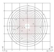
Efficiency Coordinate System Total Flux Maximum Value 62.72 lm/W CG 8643.26 lm 1266.82 cd
