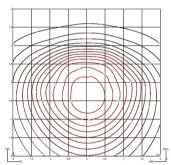
Efficiency Coordinate System Total Flux Maximum Value 58.04 lm/W CG 186 lm 510.94 cd
