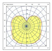
Efficiency 46.61 lm/W Coordinate System CG Total Flux Maximum Value 186.24 cd
