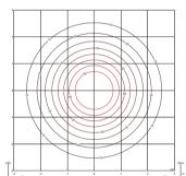
Efficiency Coordinate System Total Flux Maximum Value 56.12 lm/W CG 1664.84 lm 365.39 cd
