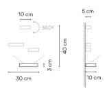
25 Beige D1 test ral 93 White **RAL 9003** 2700 K / 3500 K LED temperature color 0-10V Dimming Surface Canopy Instalation type Body: Aluminum Materials Diffuser: Borosilicate Lid: PC- Polycarbonate Reflector body: Foamed PVC 1x LED 9W 350mA Light source
