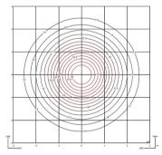
Efficiency Coordinate System 51.19 lm/W CG 565.65 lm **Total Flux** Maximum Value 270.71 cd
