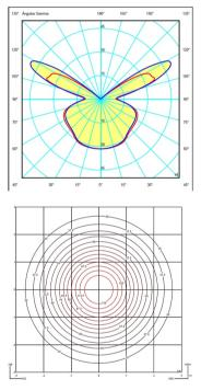
Efficiency Coordinate System Total Flux Maximum Value 38.37 lm/W CG 263,64lm 53,87cd
